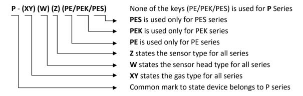
P Series designed with SH20 or SH30 Sensor Head + Junction Box P series naming schema is "P - (XY) (W) (Z)" Key code: P - \*\* (2 or 3)\*
